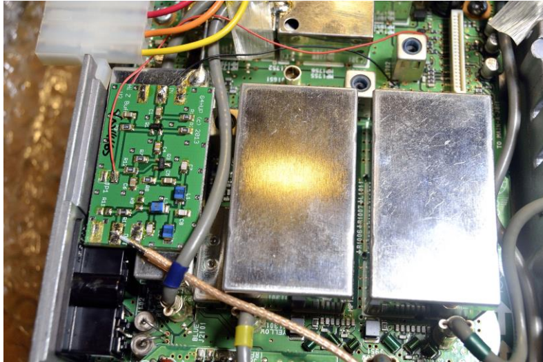
Fig 2 – Location of PAT inside IC756 Pro III
