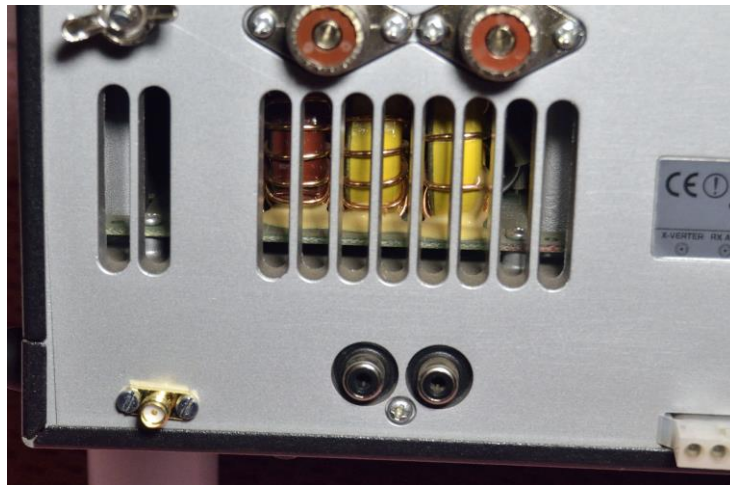
Fig 1 – position of SMA connector on rear panel
