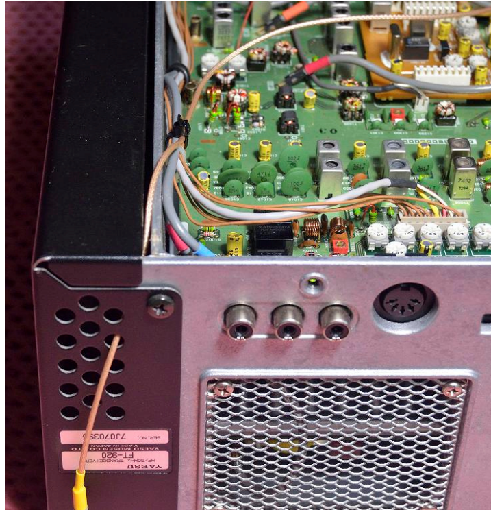
Fig 3 – Output cable routing from the FT920, over the chassis wall, and secured with tie-wrap to existing cable form
