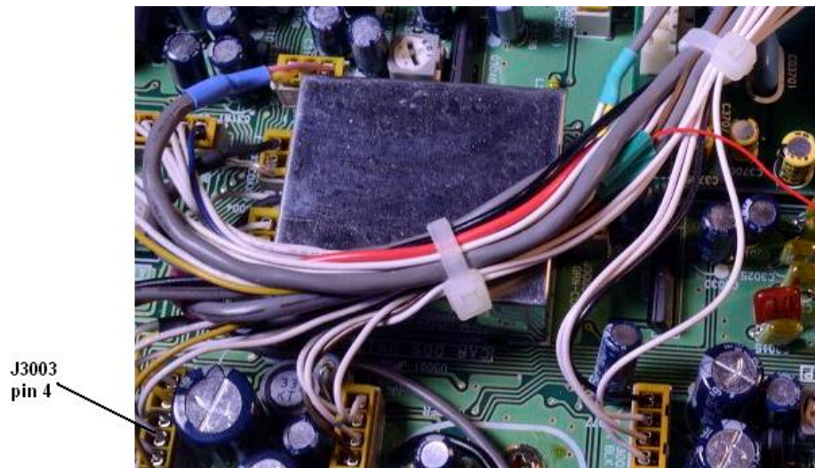
Fig 5 – Power (Vcc) connection at J3003
