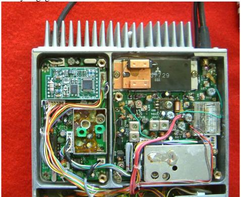
FTS-8px Installed in the FT-2700RH
