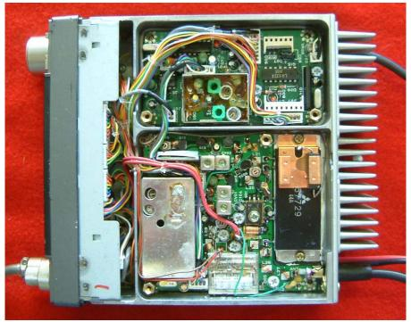
FT-2700RH Transceiver with the Dummy Board Removed.
